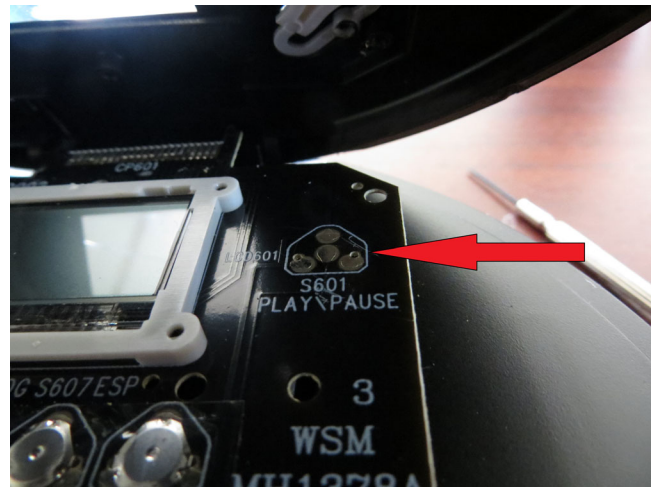
Figure 1. A close-up image of the exposed upper integrated circuit board of a CD player (INSIGNIA NS-P4112; INSIGNIA Products, Richfield, MN). When the 4 contact poles (indicated by red arrow) associated with the play button are connected by an electrically conductive medium, the unit begins playing.
